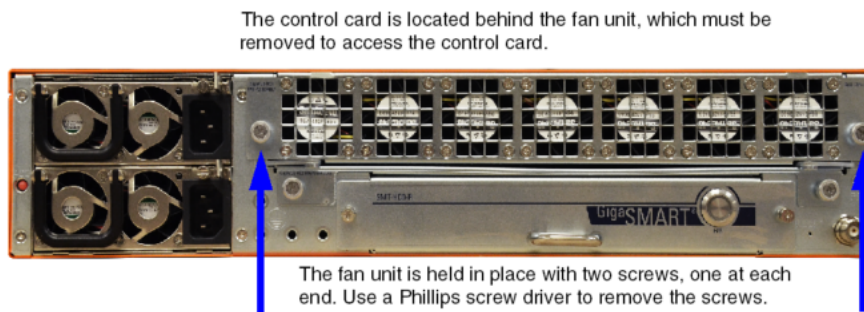
Figure 1 Replacing a Control Card
